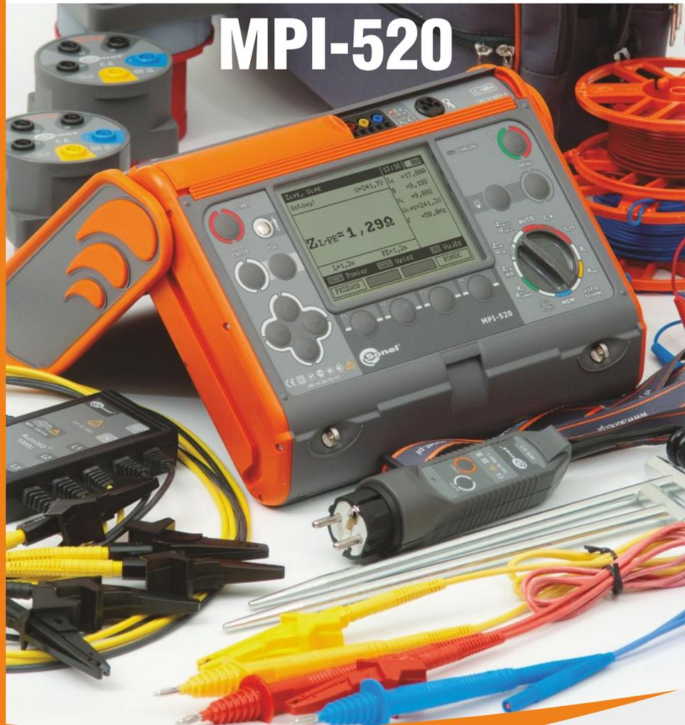
The MPI-520 multifunction meter is dedicated to perform diagnosis of electrical installation according to IEC 61557 standards. Digital meter MPI-520 is designed to measure impedance of a short circuit loop also without triggering RCD, parameters of RCD, insulation resistance, earthing resistance, continuity and also for phase sequence testing. Furthermore it is used for measurement of AC voltage and current, frequency and power.
